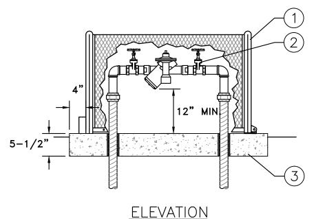
1 GUARDSHACK ENCLOSURE MODEL GS-3 WITH FROST GUARD FG-3, MOUNTED TO CONCRETE PAD. INSTALL PER MANUFACTURER'S RECOMMENDATIONS.
