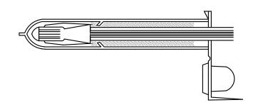
STEP 4: POSITION WIRES IN WIRE CHANNELS AND CLOSE INSULATOR TUBE COVER.
