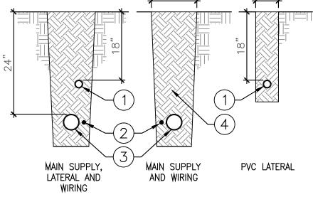
ACCORDANCE WITH MANUFACTURER'S SPECIFICATIONS. MAINTAIN MIN. 4" SPACE BETWEEN PARALLEL PIPE LINES AND 6" VERTICAL SPACE BETWEEN MAIN LINE AND LATERAL LINES. WIRING AND MAIN LINE TO BE AT SAME MIN. DEPTH OF 24".
